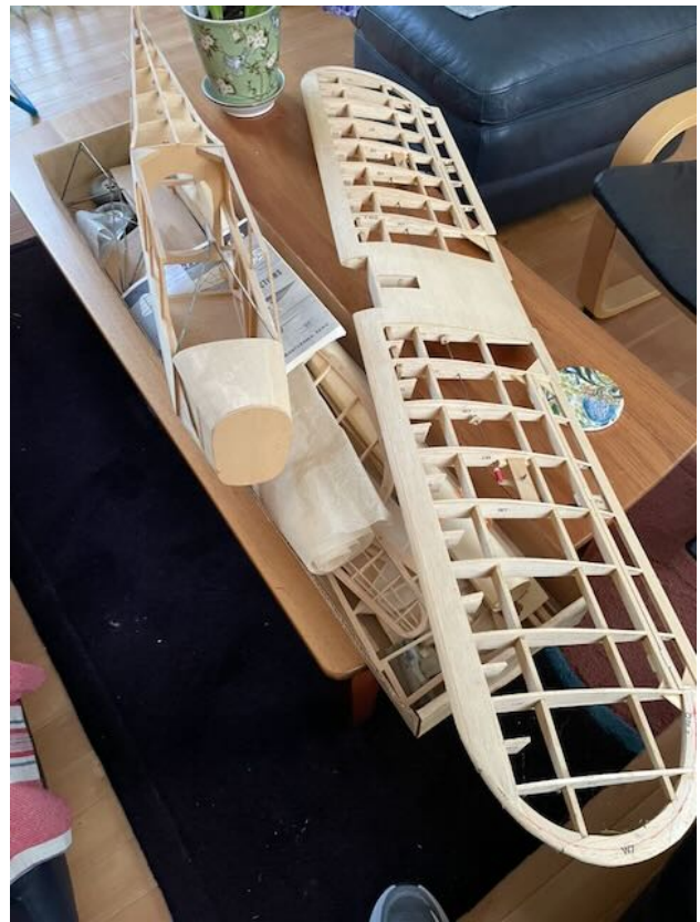
SIG Clipped Wing Cub fuse, wing, horizontal stab and rudder mostly built. some wood and plans in box
