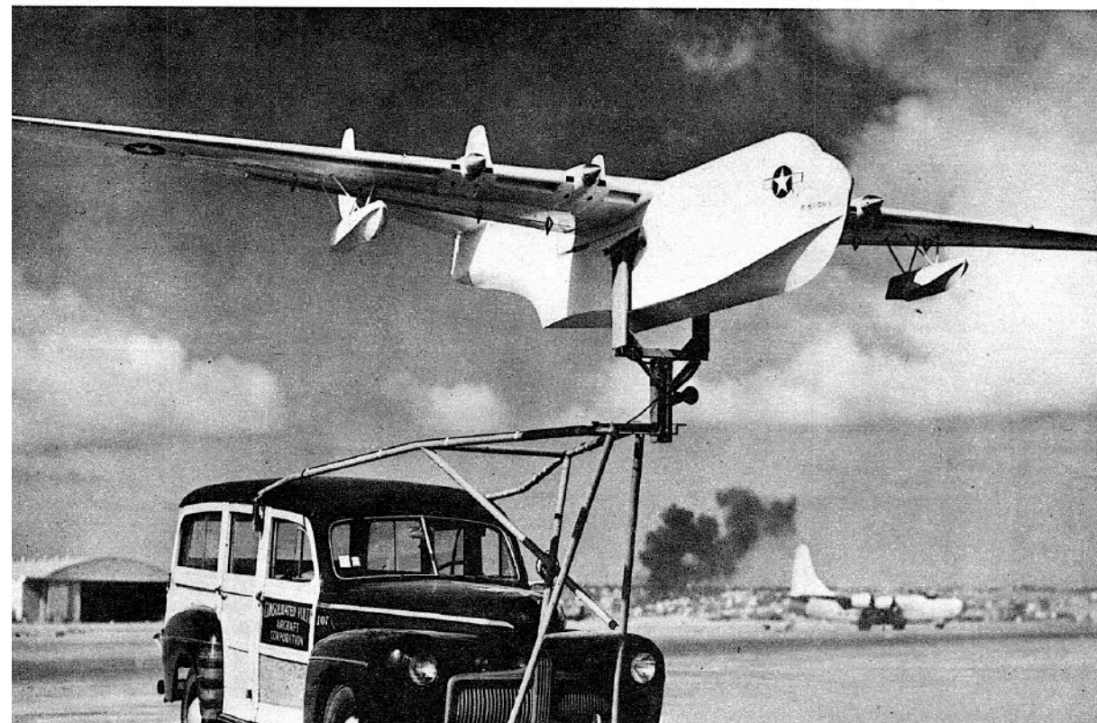
● This aerodynamic test setup of scale model and car enables determination of many flight characteristics without risking flight. Car is driven into wind.
