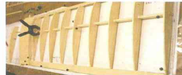
Tilt the centre section so that the lower edge of the ply brace is flat on the board and build the first panel...
