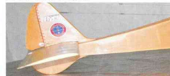
The tail control surfaces are 'sewn' hinged - the oldest - and best way.
