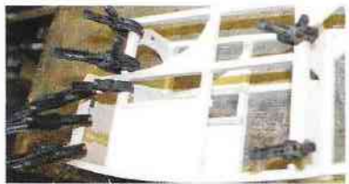
Formers are glued to the right hand side, checking for verticality, before adding the left hand side.
