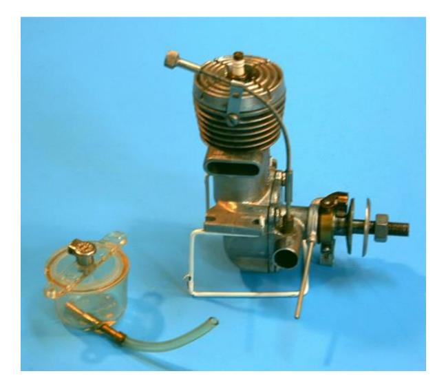
**THE CANNON 300** mentioned in the Delong article is pictured above. The cannon .358 would look identical from this angle. That needle valve setup was a good safety item to separate fingers from props and it works with surprising smoothness.
