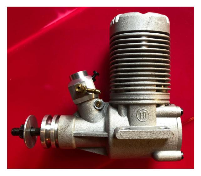
**NOT A .10 C.I.**, but a 10CC, or 60 sized MVVS engine. A good illustration of a rough finish, which some might pass up for a better looking smoother one. But – it's doubtful that there's a cooling problem even with those relatively small cylinder fins. That surface roughness might add 10% or more to the cooling area. But excess cooling in some areas isn't always a good thing, as a warm bottom end can help fuel vaporization.
