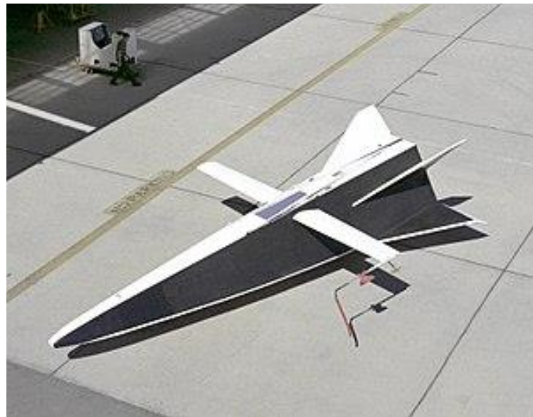
Dryden Flight Research Center E-20464 Photographed 28JUL1969 Hyper III with single-piece, pivot wing installed. Princeton sailing on ground. Daniel C. Garrabrant, one of the fabricators of the Hyper III, stands alongside. (NASA photo)
