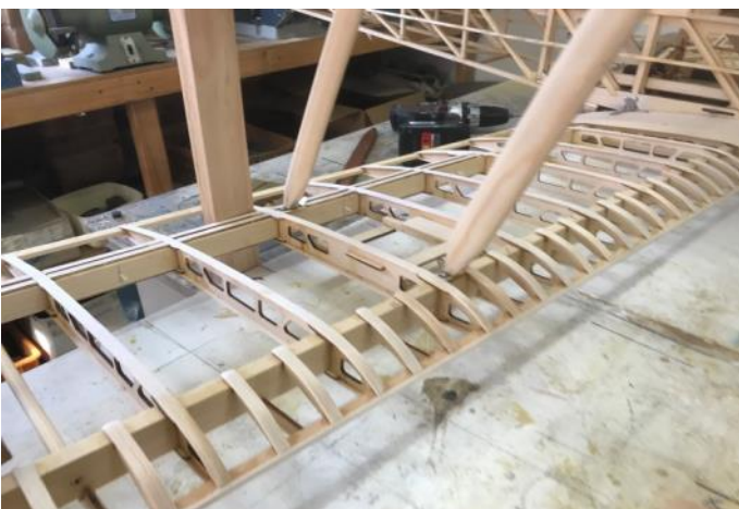
The wing structure is similar to the full size aircraft.
