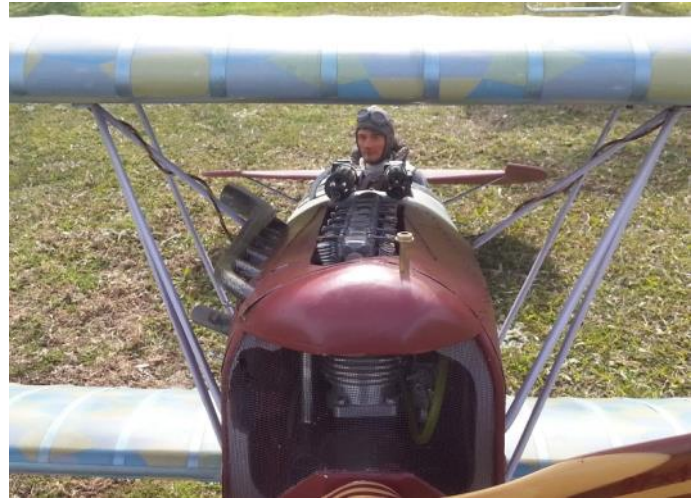
Wayne's Fokker is powered by a Moki 85cc twin in-line 4-stroke engine.
