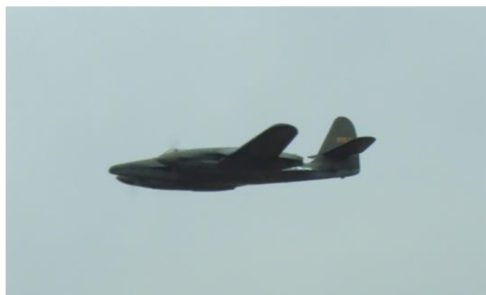
Initial test flights of the Moonbat with the undercarriage down were successful but further flying showed that the rearward retracting tricycle undercarriage had a significant effect on the centre of gravity when the wheels were up and additional nose weight had to be added to improve balance in flight.
