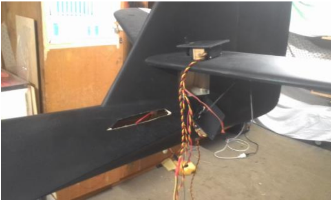
Elevator and rudder servos are at the back of the model but the long engine nacelles maintain correct balance.
