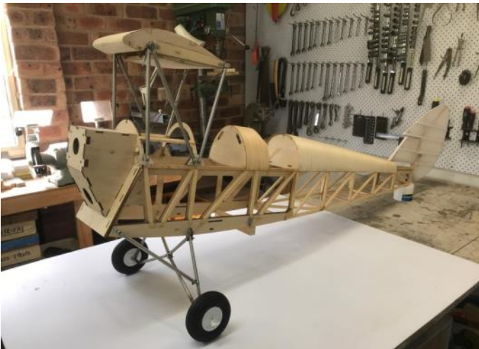
Tiger Moth fuselage. Good metal work supplied for the u/c and top wing mount.
