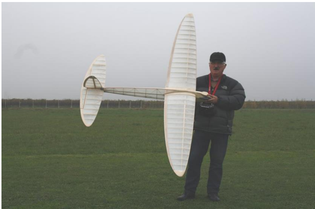
An enlarged, electric powered, radio controlled version of Luigi's 1946 model built by Rover Mersecchi.
