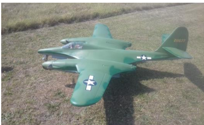
Initial test flights of the Moonbat with the undercarriage down were successful but further flying showed that the rearward retracting tricycle undercarriage had a significant effect on the centre of gravity when the wheels were up and additional nose weight had to be added to improve balance in flight.
