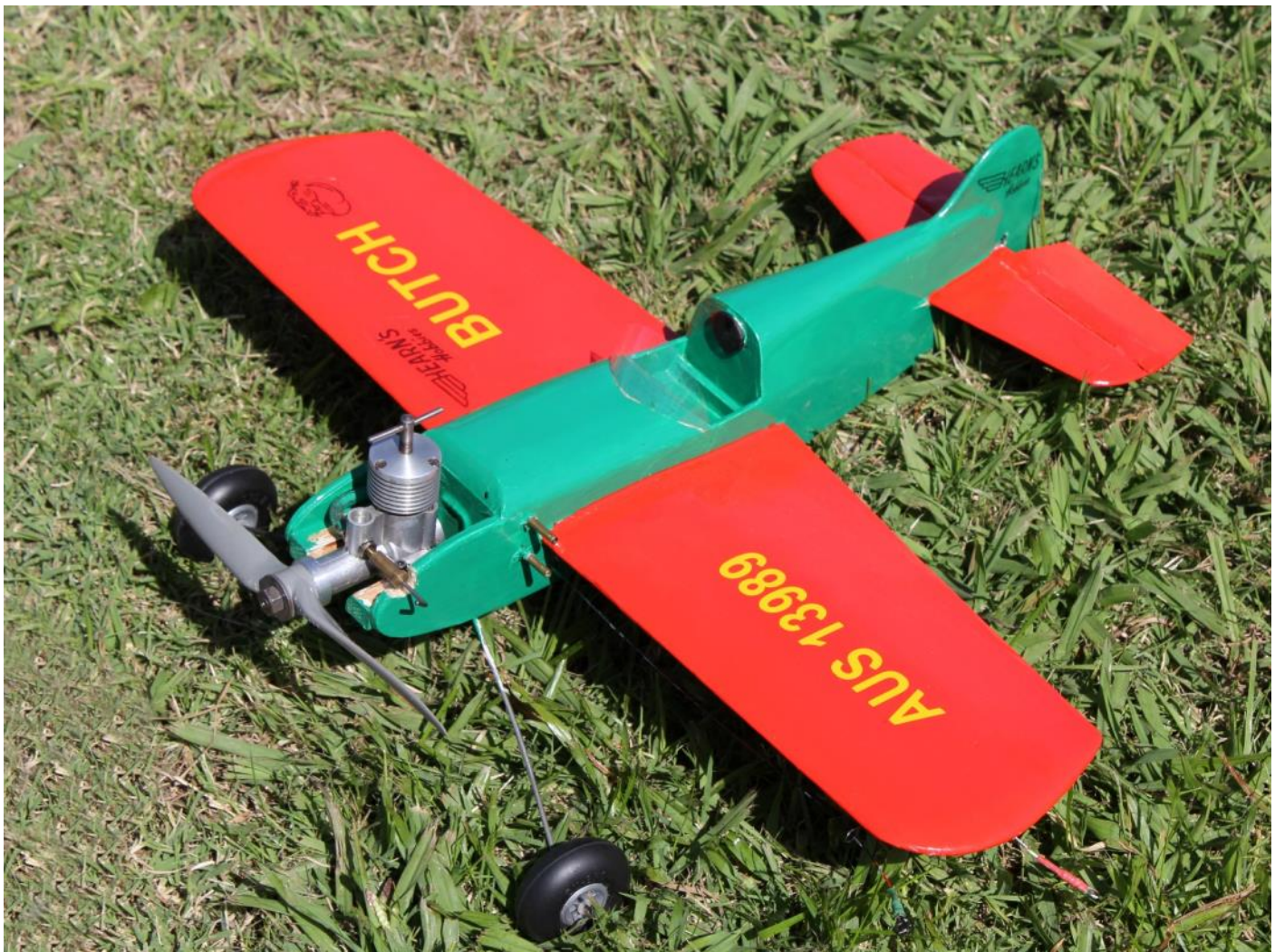
A "Butch" model built by Frank Grassham and powered by a Taipan 1.5cc diesel at the 2020 All Australian event.
