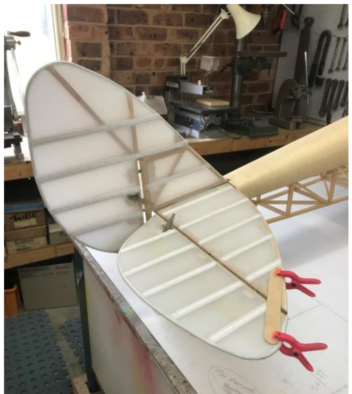
Tailplane, fin and rudder construction is near scale. Covering is SIG Koverall.
