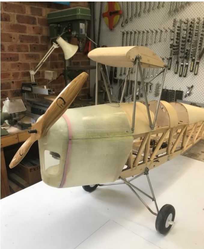
The cowl is fibreglass rather than the more common plastic moulding.
