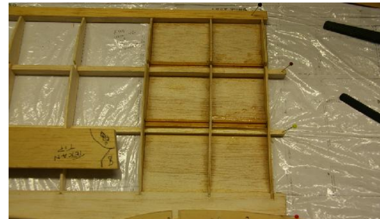
Shows bottom rails epoxied in place.
