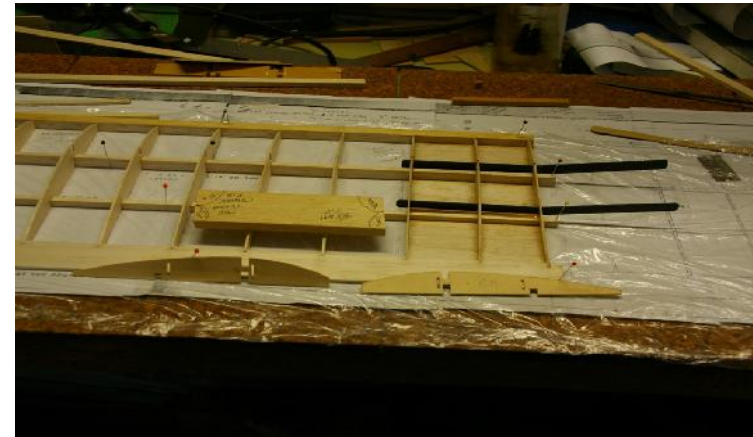
Wing joiners installed into ribs.
