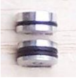
Drone diesel contra pistons. Top original Aerodyne with single O ring. Bottom contra with two O rings.
