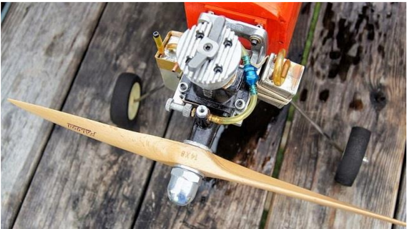
Drone with Intake Restrictor For Texaco. Two fuel tanks. One on the right in the photo for warm up. The one on the left is a Uni-flow, for smooth fuel flow.
