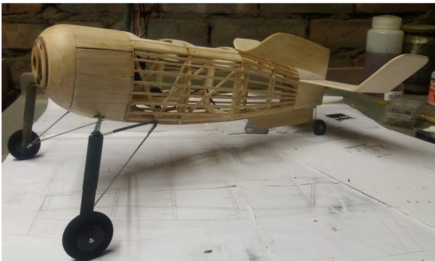
MK11 under construction
