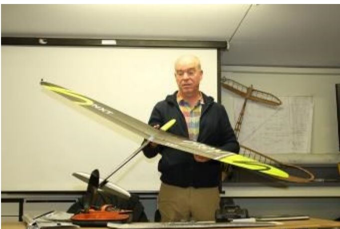
Doncaster MAC member Dan Davies presented his discus launch glider, an ARF model constructed largely from carbon fibre and manufactured in Eastern Europe.
