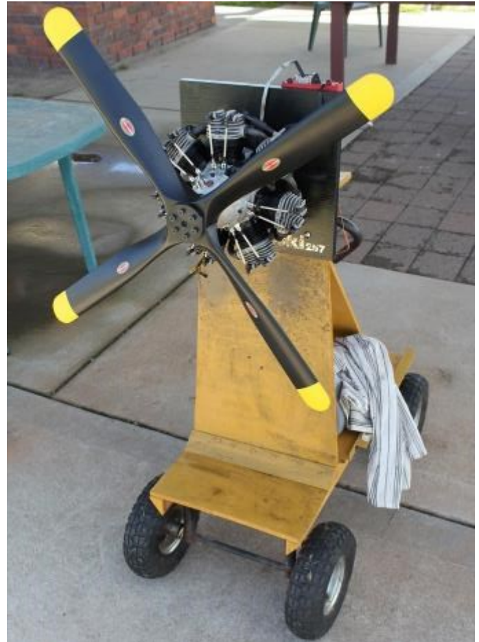
David Chivers gave himself a nice Xmas present with this Moki 257cc seven cylinder, four stroke, radial engine.
