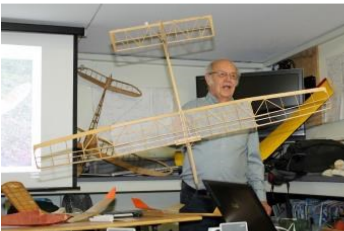
Greg Stanfield had a collection of early gliders on display including this ready to cover framework of a lightweight towline model.
