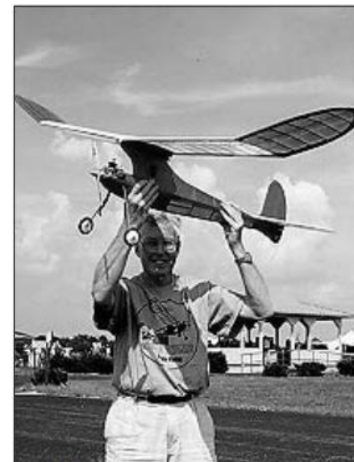
SAM Champs, Muncie, USA, August 2002 Don Howie holding the Brogini "Stardust Special" owned by John Hatch of Canada. Long wing version, 585 in 2 wing, PAW .19 diesel for A Texaco. 11x4 Topflight power point prop, Profilm (Oracover). In front of R/C area. Bitumen roads & surfaces contest sites.
