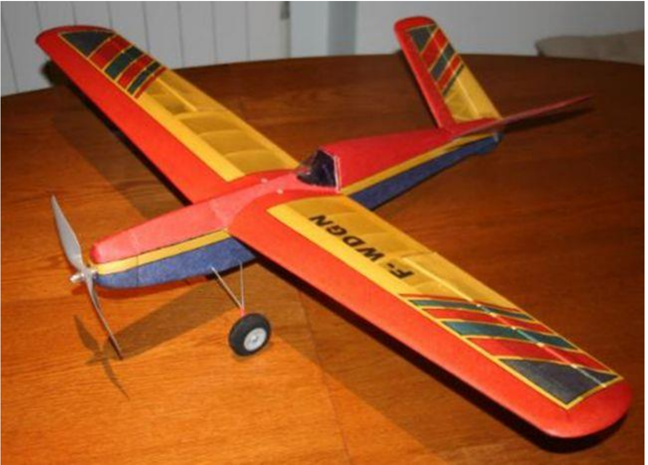
(Above) Finished 2x "Widgeon", Esaki Liteflite yellow, red and blue, nirate dope
