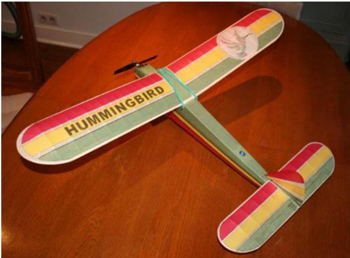
(Above) Paul Plecan "Hummingbird" with RET R/C and 50 watt electric outrunner, AUW 7.5 oz
