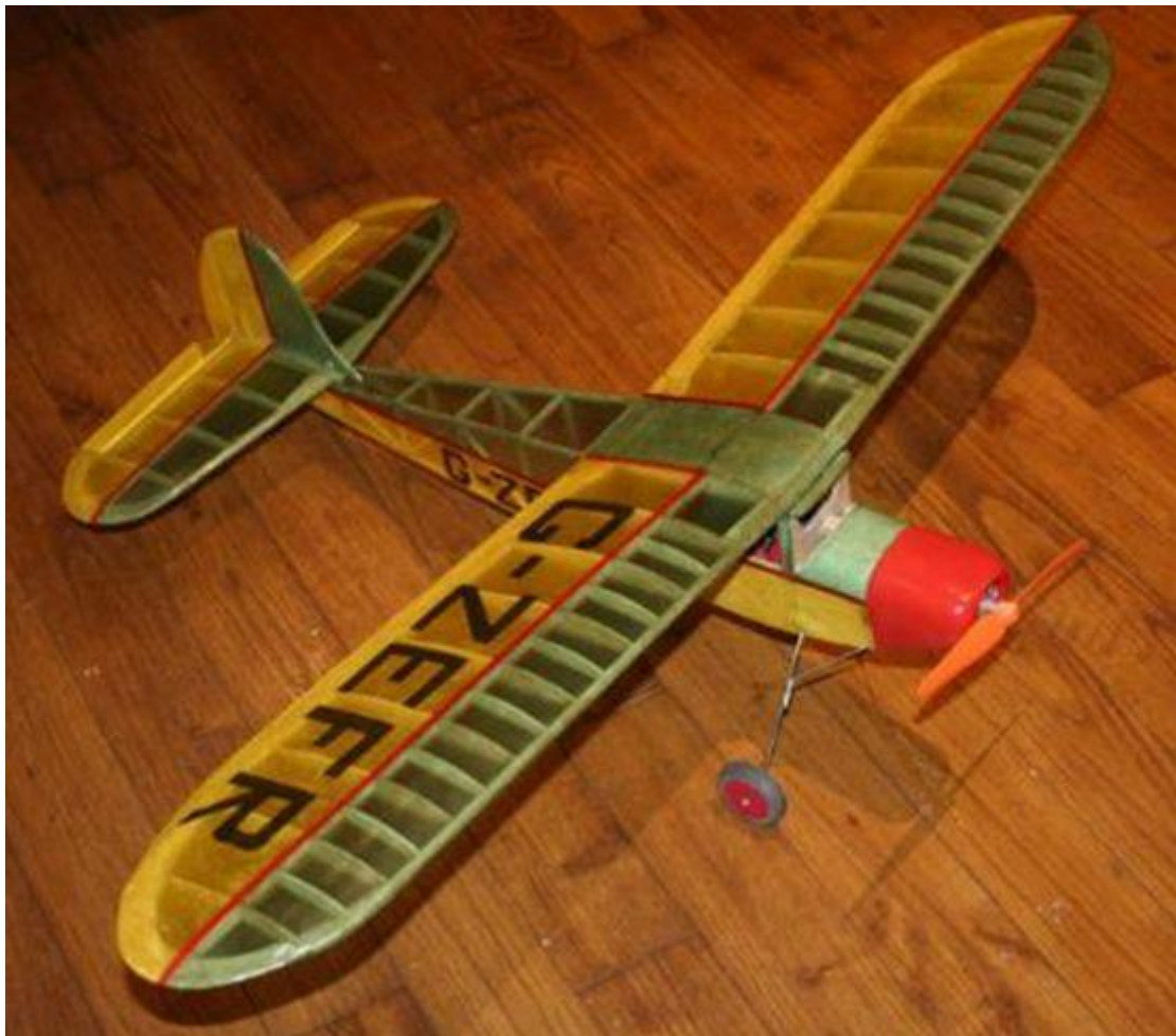
(Above) Frog "Zephyr" 60 watt outrunner powered RET R/ model, A UW 9 ounces. Notice that the WBPU gives a rather more transparent finish to the Esaki than dope does.
