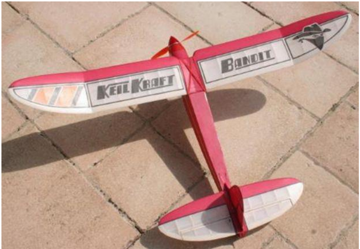
(Above) Completed electric R/C "Bandit" finished in white and coloured Esaki Liteflite over the doculam using nitrate shrinking dope. AUW 14 ounces, 160 watt outrunner.
