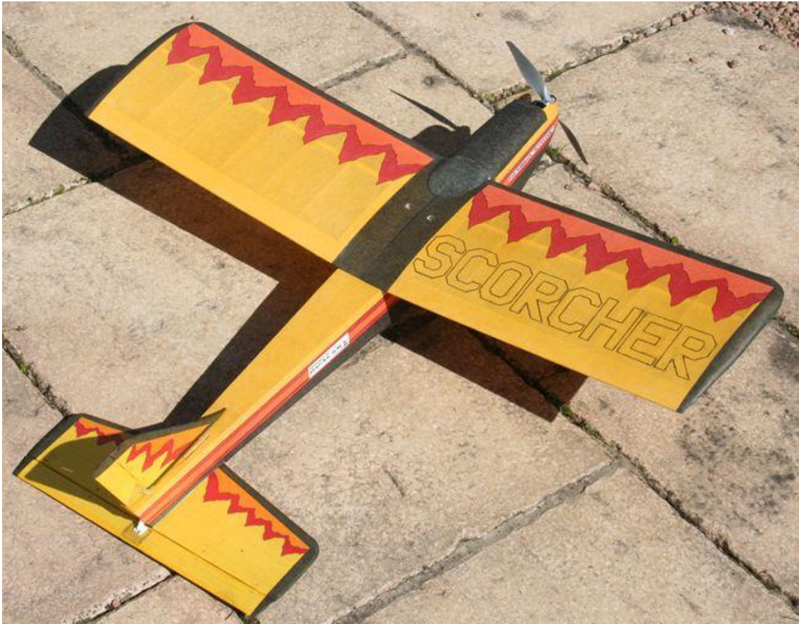
(Above) Finished "Scorcher", heavy weight yellow Modelspan on wing with colour trim of Esaki Liteflite overlaid, nitrate dope finish.
