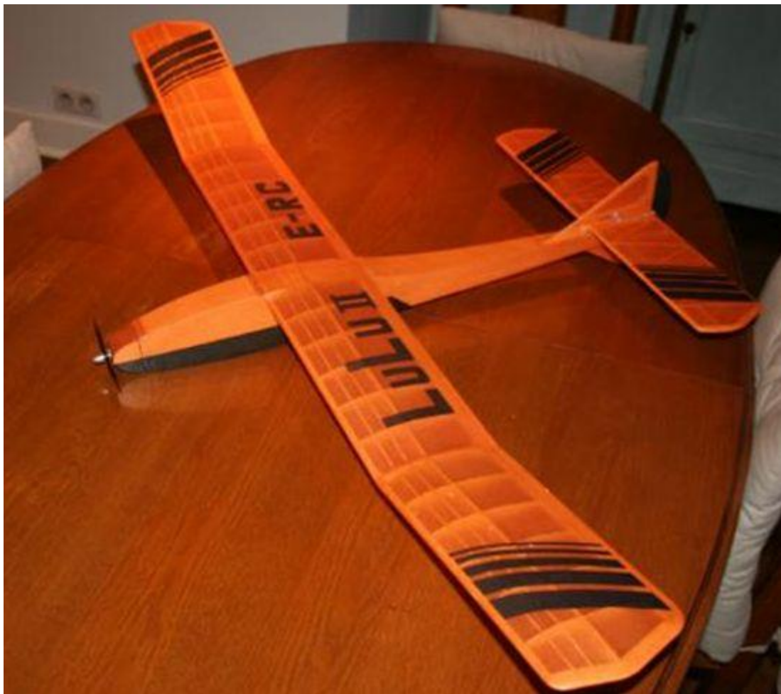
(Above) Electric R/C version of John Barker's famous Lulu II, Esaki Liteflite over 5 micron mylar, AUW 10.5
