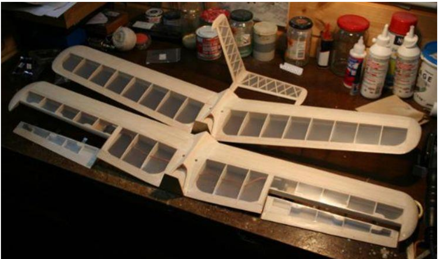
(Above) "V" tail and alternative aileron and RET wings for double size Frog "Widgeon" covered in 37 micron doculam
