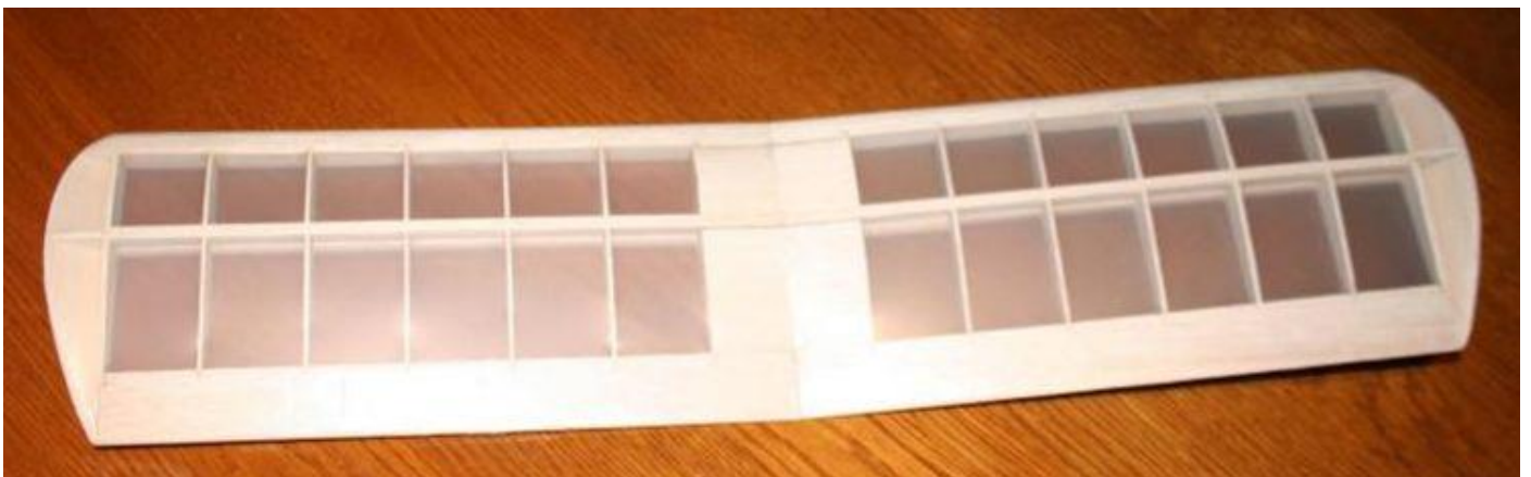
(Above) Eric Clutton "Sharkface" wing covered in 37 micron Doculam
