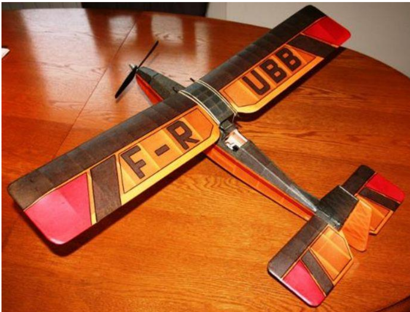
(Above) Electric R/C REAMT version of Rubberdub seem earlier with mylar applied, now finished in Esaki Liteflite. AUW 4.5 ounces
