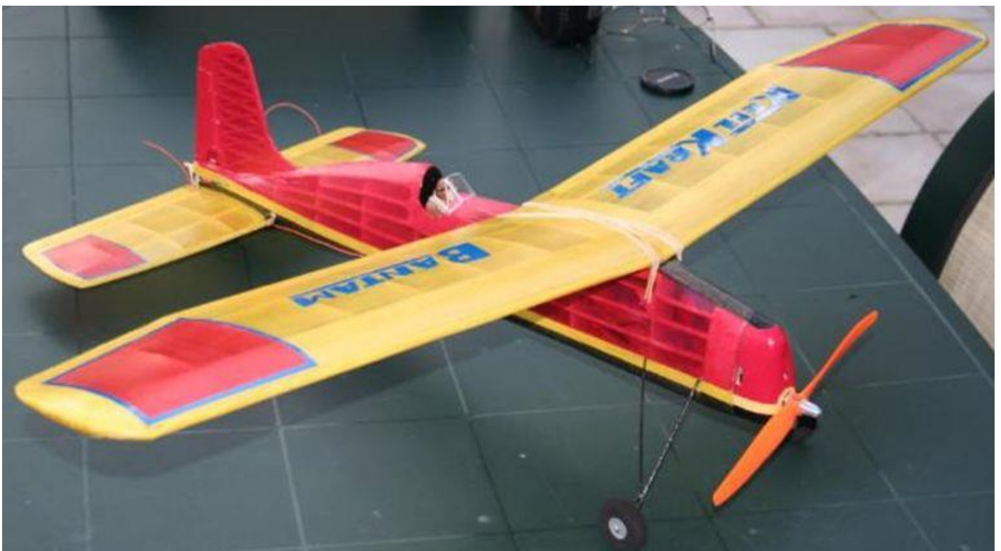
(Above) KK "Bantam", 120 watt electric RET R/C, AUW 12 ounces. Light Modelspan and WBPU
