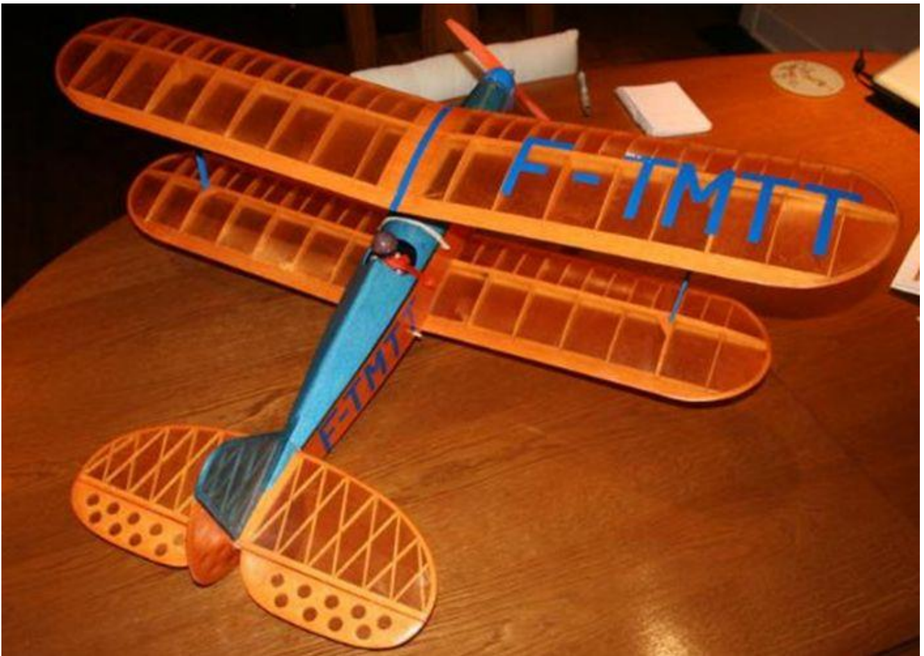
(Above) Double size Frog "Tomtit" electric R/C model, 140 watt outrunner motor, auw 16 ounces covered in Esaki Liteflight orange over 5 micron mylar using WBPU varnish (actual brand is W3W gloss) Still flying after 7 years and over 250 flights – but a bit more faded than this now!
