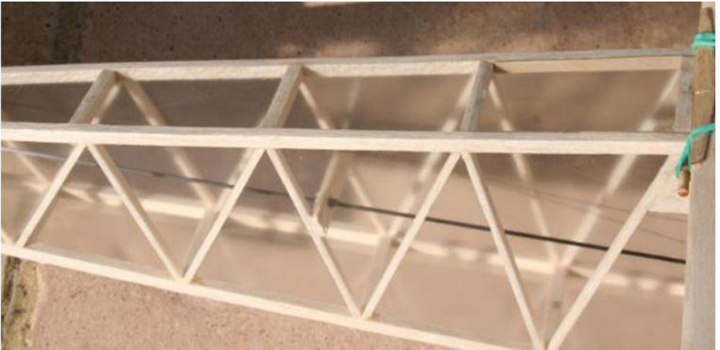
(Above) KK "Bandit" rear fuselage covered in 37 micron document laminating film, note that film is almost completely transparent after shrinking, before this the adhesive gives it a translucent appearance
