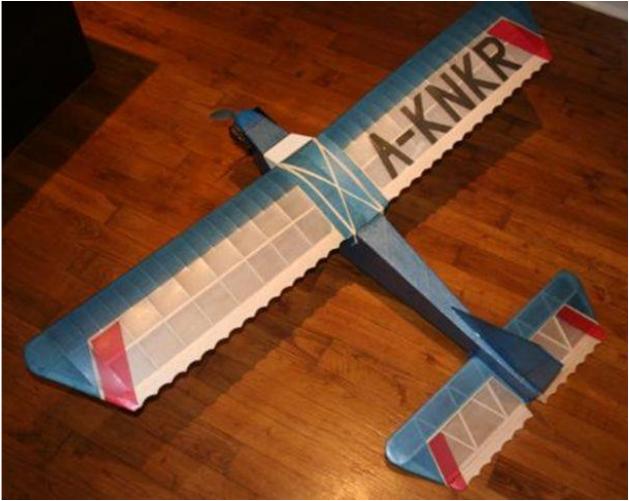
(Above) "Airknocker" after finishing with white light Modelspan tissue and Esaki Liteflite coloured trim using nitrate shrinking dope.
