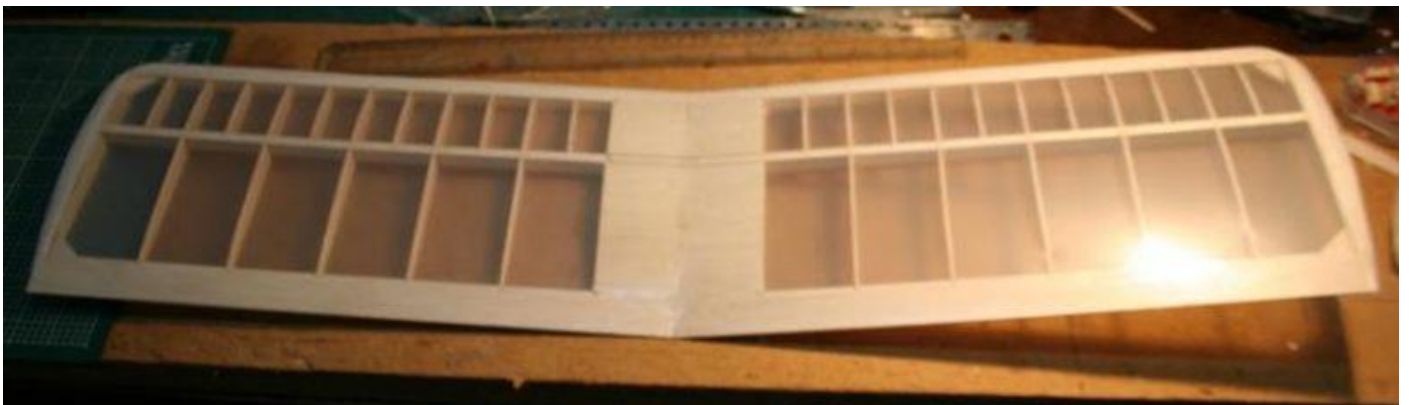
(Above) Ken Willard designed "Scorcher" wing covered in doculam
