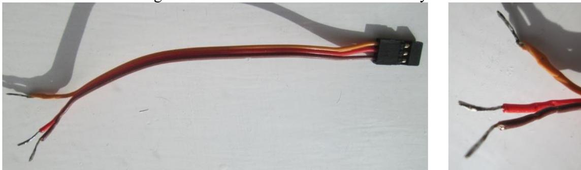
*Here is lead with bared end to modeule and other to install into the encoder board. The free ends have been soldered to make semi rigid.*
