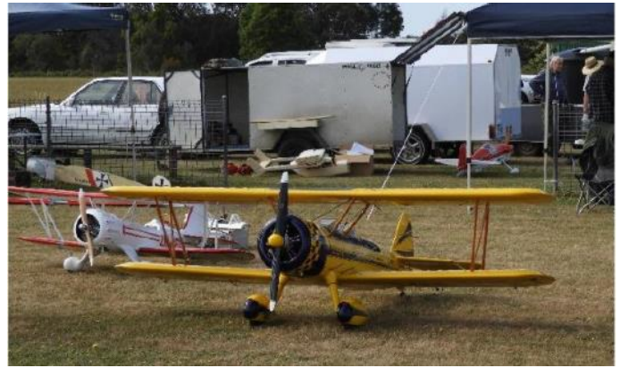
Garry Bergen's 1/3 scale Super Stearman built from a Balsa USA kit and powered by a Moki 215cc five cylinder, four stroke, radial engine.
