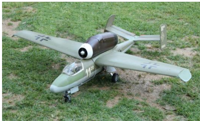
Rob Dickson's Heinkel He.162 is powered by an electric ducted fan.
