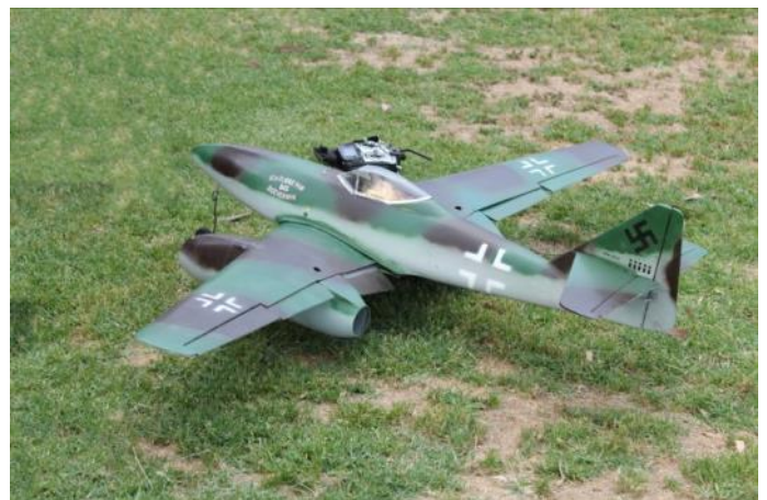
Rob Dickson's Messerschmitt Me.262 is powered by two electric ducted fans.
