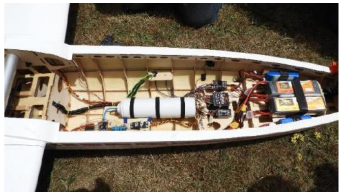
Batteries in the nose and a cylinder to store compressed air to raise and lower the power pod.
