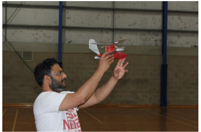
Knotting of the rubber motor limited the trimming flights of the Scheldemeeuw.
