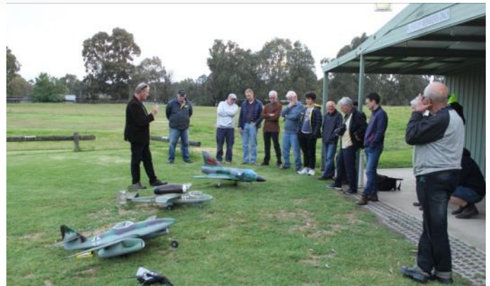
Rob Dickson describing his three model jet aircraft. The Messerschmitt Me.262 and Heinkel He.162 are powered by electric ducted fans while the Mirage III has an i/c engine at the rear with a pusher propeller.
