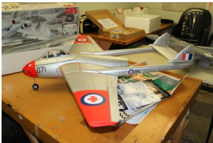
Another of Cliff's models, this ARF foam model of the DH. Vampire is powered by an electric ducted fan.
