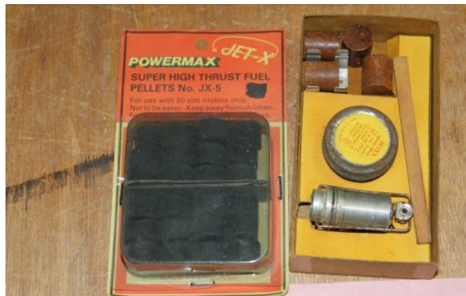
The Jetex engine was really a solid propellant rocket motor and was popular for a short time with a number of small jet aircraft kits designed to use it.
