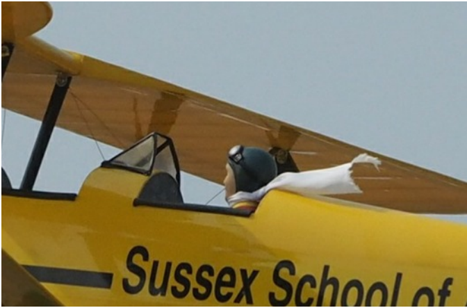
Peter Ederle's Tiger Moth is a Great Planes ARF with a 1780mm (70") wingspan. The engine is a 20cc DLE petrol that provides ample power for what Peter describes as a very pleasant flying model.
