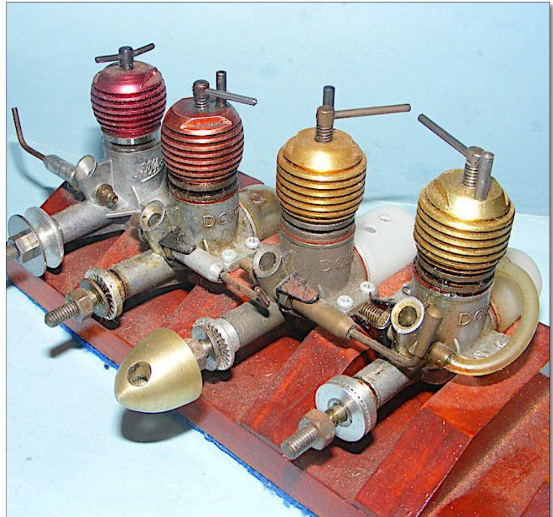
Fig 9. DC Dart production through the decades: Mk2, 'Quickstart', Performance Kits 'PK Dart Special' and the final 'Dav-Cal' yellow head Dart-notorious for breaking crankshafts
