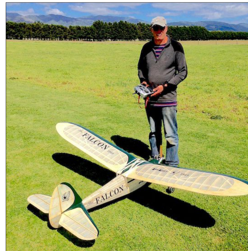
Trevor Glogau with his 96" Falcon after making two 15 minute flights for the Open Texaco Leader Board. Design is a copy of the Shershaw Cloud Cruiser with a larger fin. Trevor uses a Saito 4C spark ignition engine.
