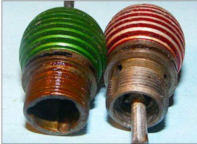
Fig 6. The Mk2 Allbon Dart cylinder (R) changed to external transfers
