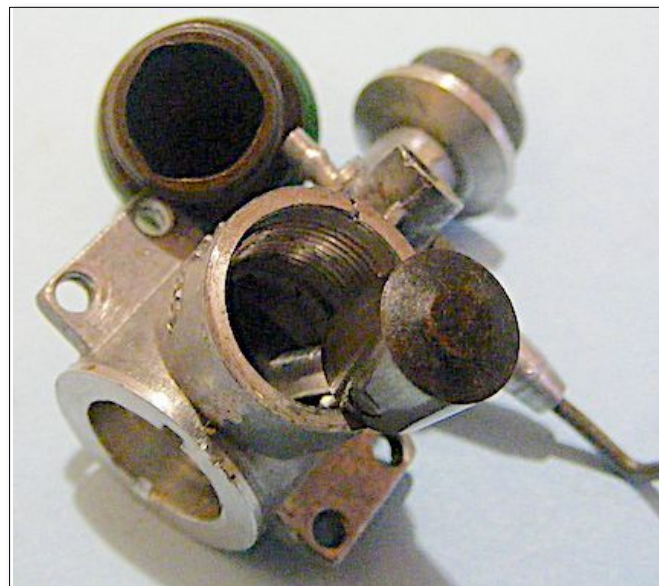
Fig 4. The Allbon Dart Mk1 series 2 changed to a conventional gudgeon pin arrangement
